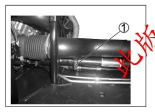
1. V-belt cooling duct check hose
