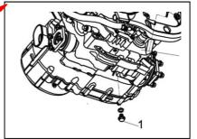
1. Engine oil drain bolt
