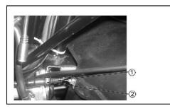
1. Brake light switch 2. Adjusting nut
