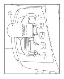
To shift from N to H or R, from L to H, from P to R, depress the button of gear selector. To shift from H to L or N, from R to N or P, it's not necessary to depress this button.
