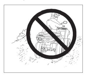
Never apply the rear brake while rolling backwards. Apply the front brake. When fully stopped, apply the rear brake as well, and shift the gear to parking.
