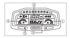
**SPEEDOMETER (2):** shows the vehicle speed. In ODO mode, press and hold SET(5) to toggle between KM and MP.
