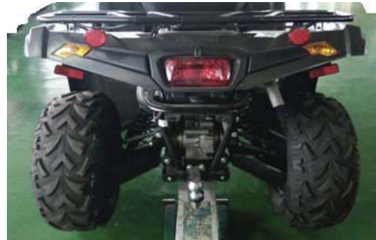
TYPICAL BACK UP POINT LOCATION
