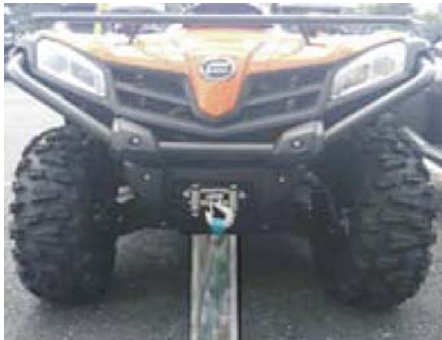
TYPICAL FRONT UP POINT LOCATION
