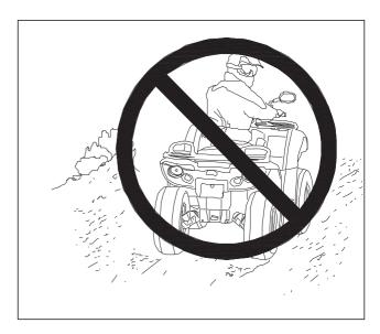
Never apply the rear brake while rolling backwards. Apply the front brake. When fully stopped, apply the rear brake as well, and shift the gear to parking.
