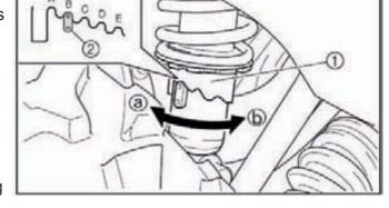
To decrease the spring preload, turn the adjusting ring in Direction (b) .
